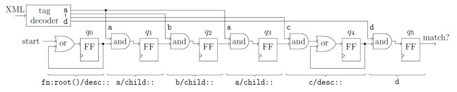
decomposing non-deterministic finite-state automata into (i) structural skeleton (logic) and (ii) reconfigurable conditions (memory)
