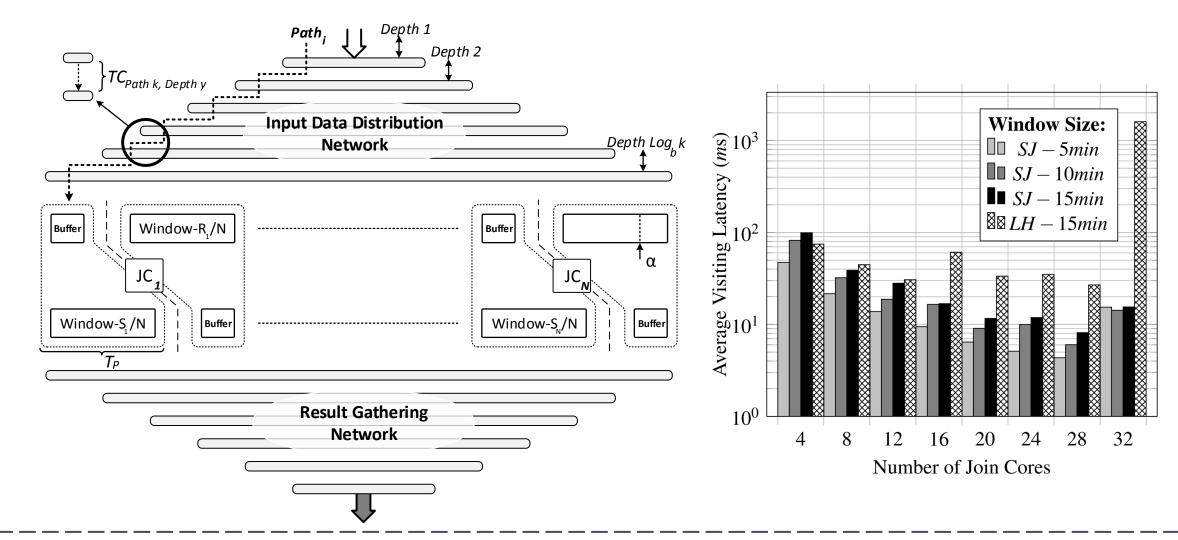
rethinking the data flow to eliminate the control flow & split the join into concurrent/independent "store" & "process" steps
