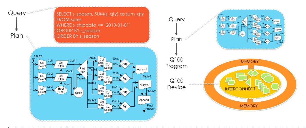
supporting arbitrary-size query given a fixed logic-budget through horizontally partitioning of query into pipelined stages
