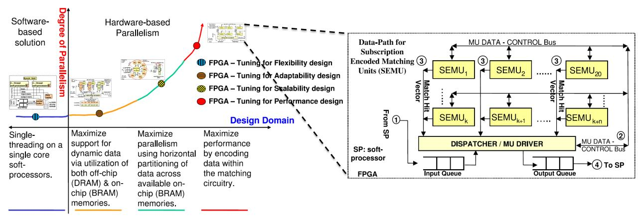
encoding each query as a custom logic block for maximum parallelism
