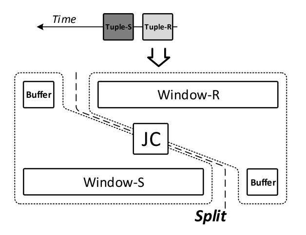
rethinking the data flow to eliminate the control flow & split the join into concurrent/independent "store" & "process" steps
