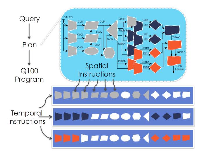
supporting arbitrary-size query given a fixed logic-budget through horizontally partitioning of query into pipelined stages
