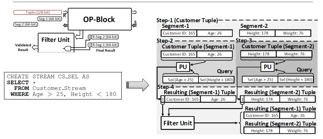
supporting arbitrary-size schema given a fixed wiring/routing-budget through a vertically partitioning of query and data
