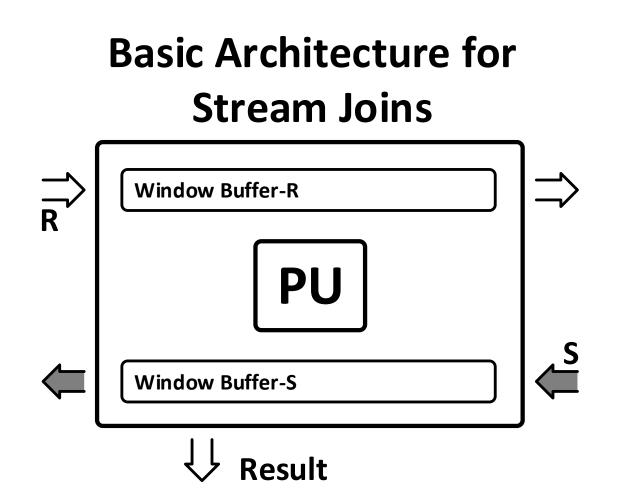
rethinking the data flow to eliminate the control flow & split the join into concurrent/independent "store" & "process" steps
