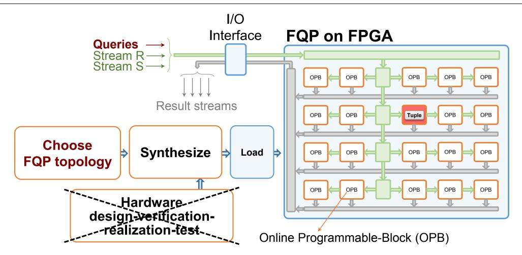
constructing complex queries from composable reconfigurable logic blocks, where composition itself is reconfigurable
