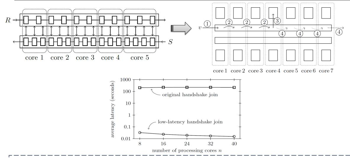
introducing bi-directional data flow to naturally direct streams in opposite directions to eliminate complex control flow
